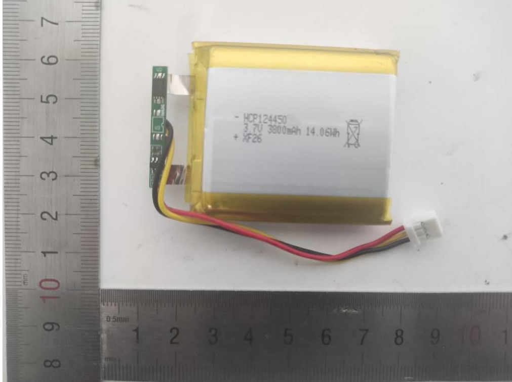
Figure 3 Internal view of battery
