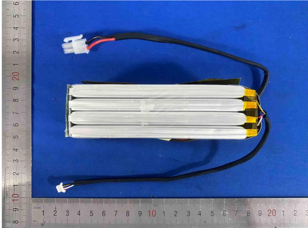
Figure 3 Internal view 1 of battery
